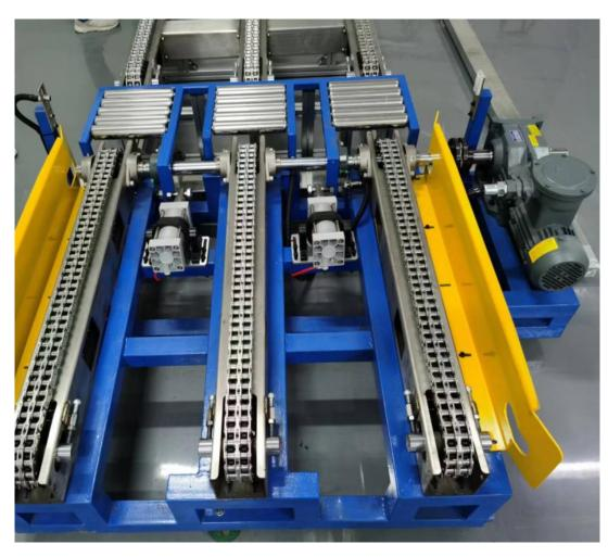
Ensures high precision at loading and unloading Stainless stee rollers, ATEX type motors
